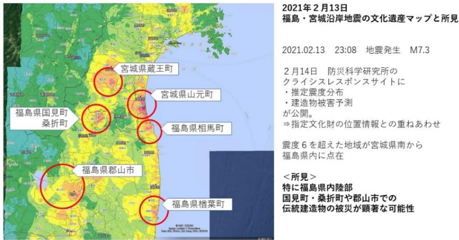
Fig. 22 Estimated seismic intensity of an earthquake of February 13 th , 2021 and location of cultural heritages [CTOC19]
