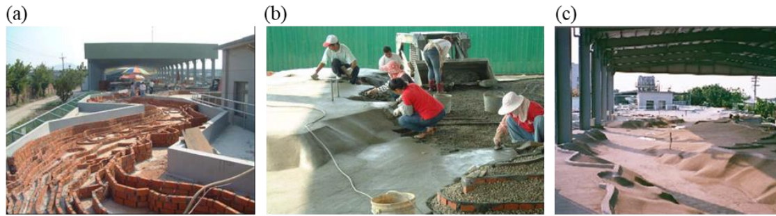
Figure 3.20 The Shihmen Reservoir physical model construction uses (a) brick for contour setup and (b) cement mortar and gravel for reservoir bed and terrain construct. (c) the completion of the physical model.
