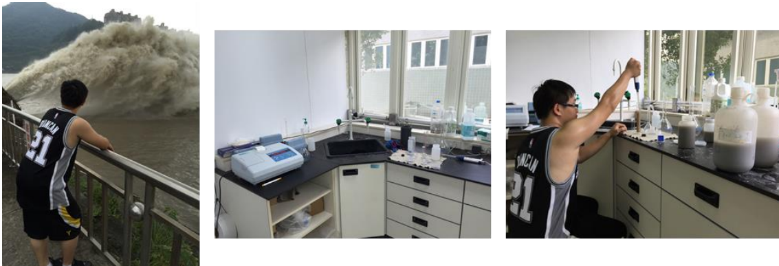
Figure 3.9 Taking the turbidity flow sample and measuring the turbidity and sediment concentration by using turbidity meter and gravimetric analysis.
