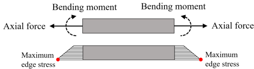
Fig. 4-18 Illustration of internal force and maximum edge stress of beam element
