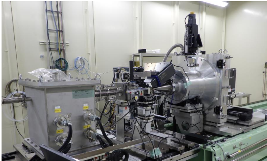
Fig. 2.8.7 A photograph of the SAXS-CT experimental set up at BL03XU in Spring-8
