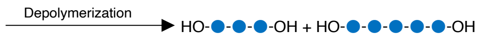
Figure 3.14. Schematic illustrations to describe the POM copolymer and oxidative decomposition by VUV irradiation within 10 min.
