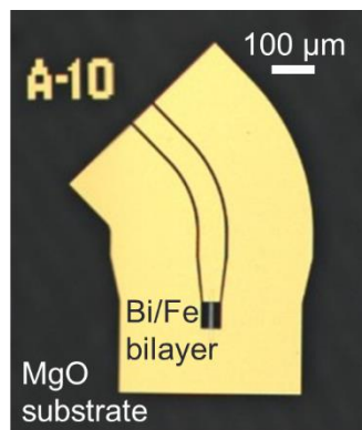
Figure 5-5. Magnified image of measurement device, consisting of Bi/Fe channel (gray rectangle located below the centre) and waveguide (gold region)
