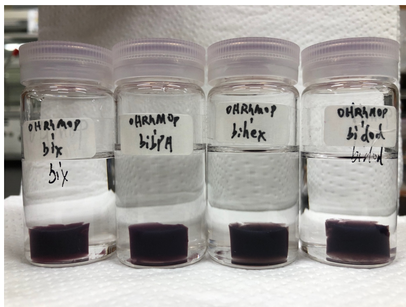
Figure 3-8. Photos of gel samples of (a) (\text{ONa})_6\text{RhMOP-bix} , (b) (\text{ONa})_6\text{RhMOP-bibPh} , (c) (\text{ONa})_6\text{RhMOP-bihex} and (d) (\text{ONa})_6\text{RhMOP-bidod} .
