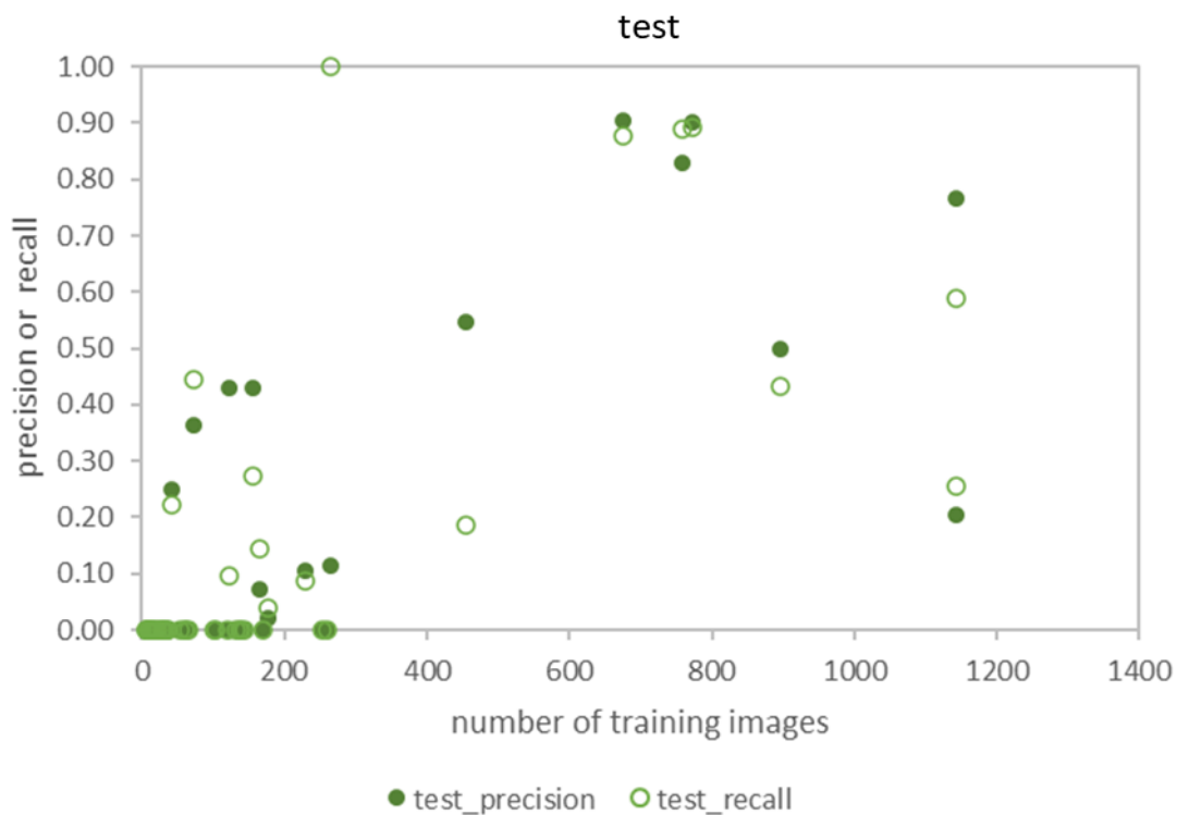
Figure 3.11 Relationship between precision or recall accuracy and number of training images. From top to bottom, the accuracy of validation 1, validation 2 and the test.
