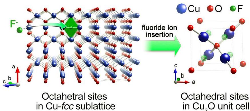
Figure 4.12 Octahedral sites in the Cu- fcc sublattice and the continuous channels along [011] direction for “topotactic Cu 2 O” hypothesis.
