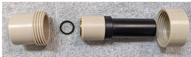
Figure 3.1. A schematic illustration of the working electrode
