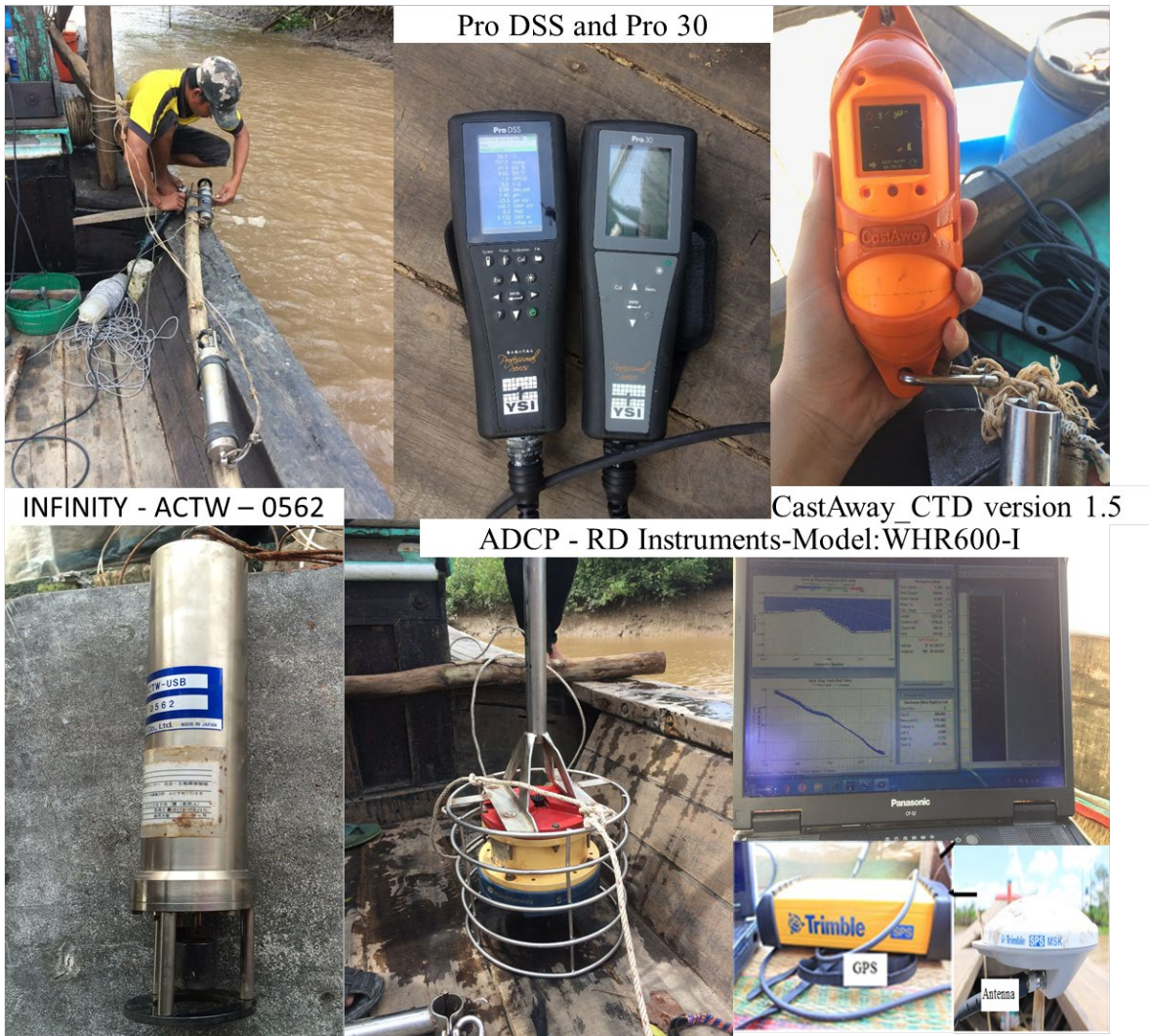
Figure 3.4 The measurement instruments used in the field survey
