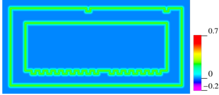
Figure 3.3: Initial map m(0) (conventional likelihood field map) in simulation
