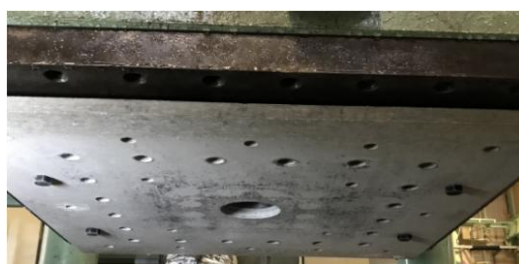
Figure 2.6 Heat insulating plate installed on the top loading interface
