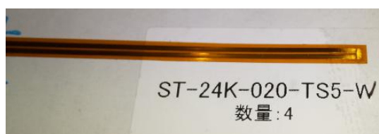
Figure 2.7 Thermocouple used in the test
