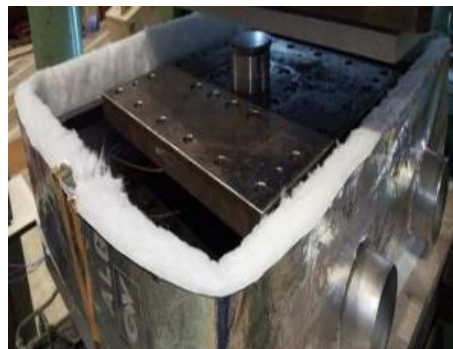
Figure 2.3 Bearing specimen placed in the insulation chamber
