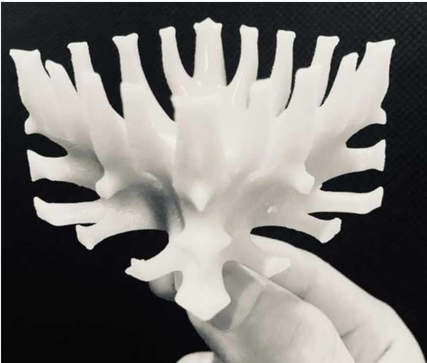
FIGURE 4.23: Resin-based 3D printed prototype, cf. 3D case #2.
