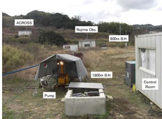
Photo 1 Water-injection experiment in 2000 at the borehole observation site of the Nojima fault
