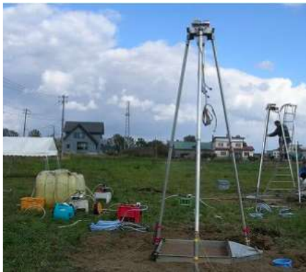
Photo 9 Field sprinkle equipment for infiltration
