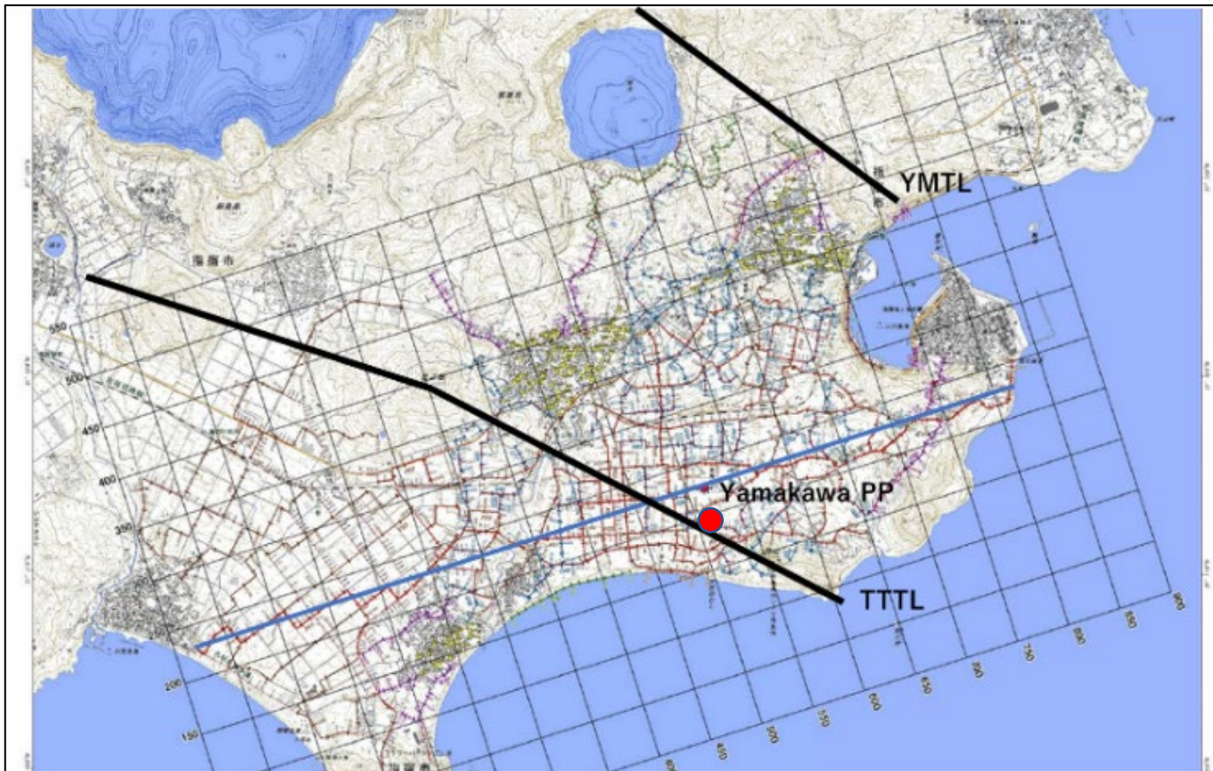
Figure 3-2. Location map of the Ibusuki geothermal area in Kagoshima Prefecture (modified from AOKI, 2018; JOGMEC, 2018). The area of 3-D seismic survey shows in coarse mesh. Two tectonic lines, TTTL and YMTL, Yamakawa PP, and the common line (in blue) of respective seismic sections of 2-D and 3-D (profile 230) are shown.
