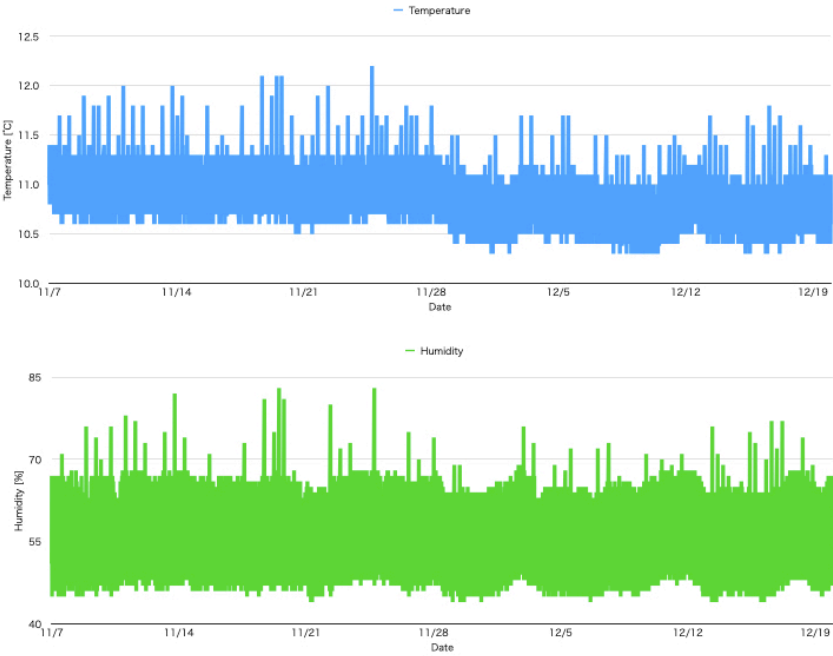
Figure 4.19: Temperature and humidity inside a cooling shelter during 2019.
