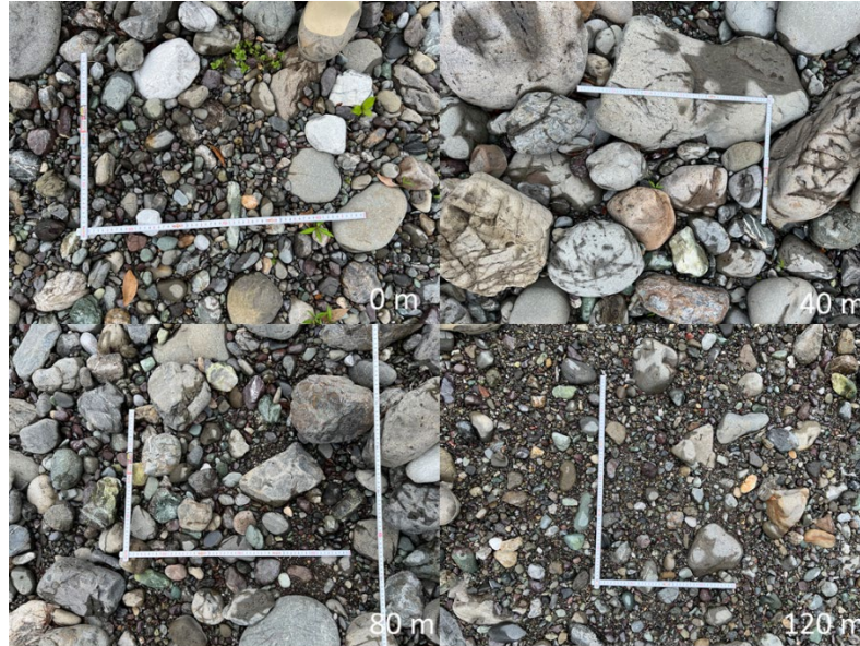
Figure 3-20 The photos of grain distribution at 0 m, 40 m, 80 m, and 120 m at gravel bar 4 in the 2022 field survey.
