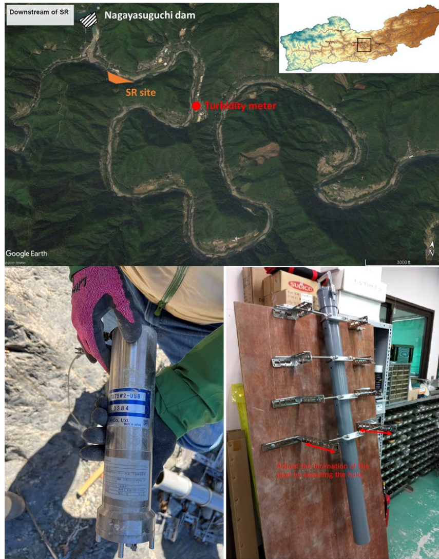
Figure 3-22 Top figure: the installed location of the turbidity meter in the Naka River. Bottom figure: the photo of the turbidity meter and the installed method.
