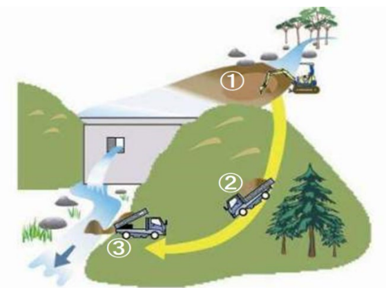
Figure 2-1 The process of SR implementation from the excavation site to the replenishment site (S. Kantoush et al., 2010).
