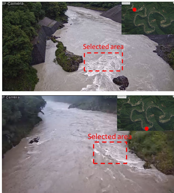
Figure 5-3 The measured locations of STIV for calibration and validation of hydrodynamics in TELEMAC-2D. The red squares represent the selected area for flow velocity calibration and validation. Top figure: Kohama. Bottom figure: Mizaki.
