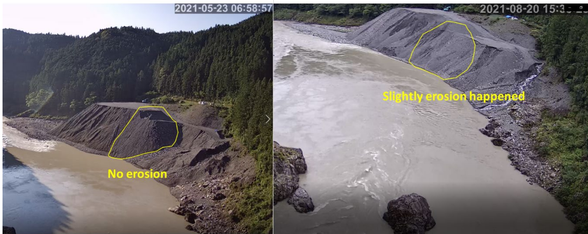
Figure 4-34 The comparison of eroded area between flood events in May and August, 2021 in the Naka River.
