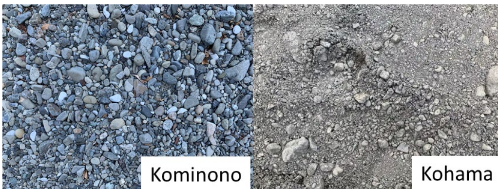
Figure 3-6 The comparison of sediment between Kominono (potential sediment source) and Kohama (current replenishment sediment)
