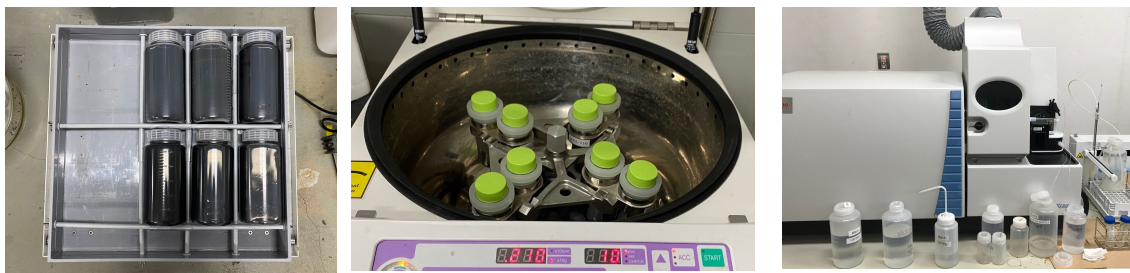
Figure 4.1: Batch leaching test steps: shaking, separating with centrifuge and ICP- AES and ICP-MS analysis
