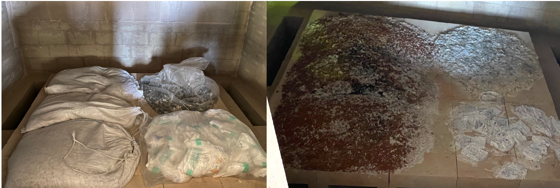
Figure 3.6: Before and after pyrolysis thermal treatment of industrial mixed plastic, soil mixed with waste and disposable diapers
