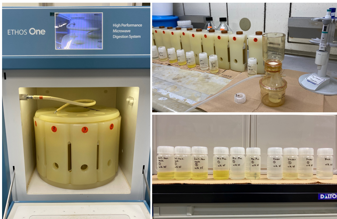
Figure 4.2: High Performance Microwave Digestion System ETHOS One, Milestone and samples
