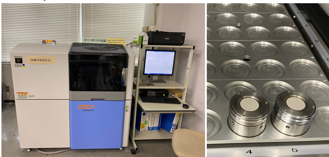
Figure 3.5: XRF instrument and analyzed samples
