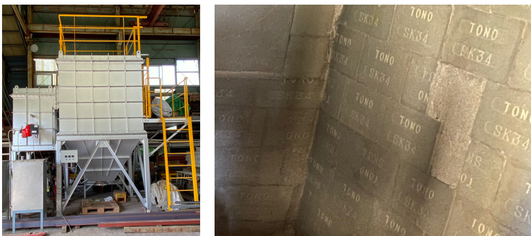
Figure 3.3: Demonstration of pyrolysis technology chamber and ceramic wall inside the chamber
