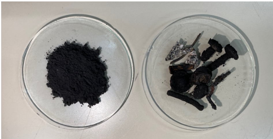
Figure 3.2: Separation of plastic and metal parts through high-temperature steaming: left –plastic, right – separated metal parts
