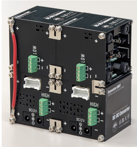
Figure 5.11: Output connection structure of fabricated dc-dc converters. Input side has no connection due to separate voltage sources.
