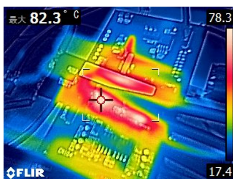
Figure 5.5: The substrate temperature at 100 W operation of fabricated converter.
