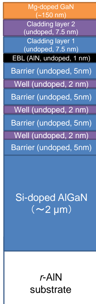
Figure 5.4: Designed r -plane LED structure which emit UVC light in this study.
