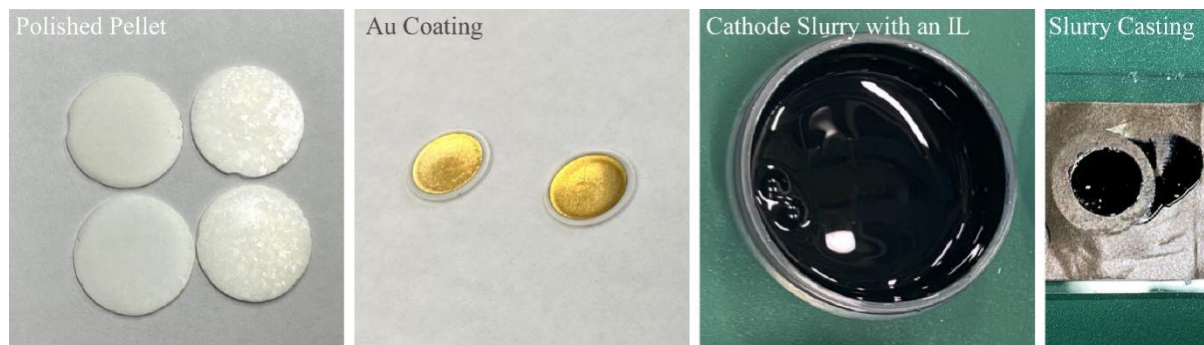
Figure 5 S1. The procedure of casting the quasi-solid-state LCO cathode slurry onto the Al-LLZO pellet's surface, Related to Figure 5.3.
