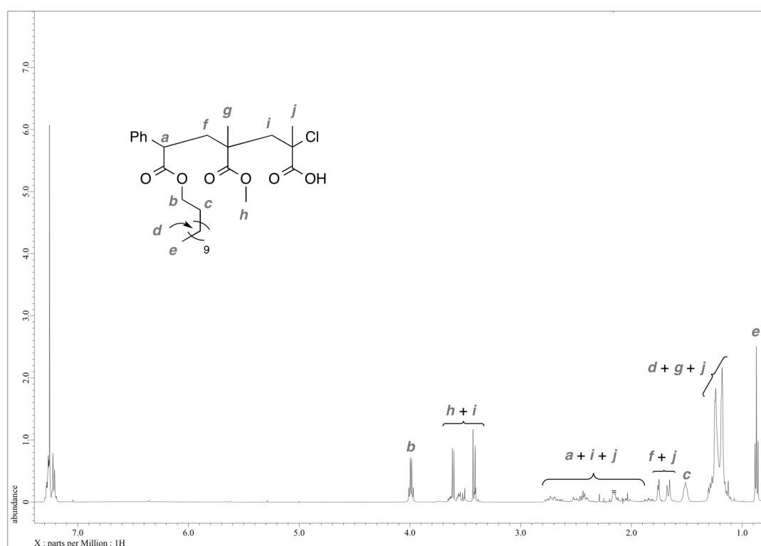
Figure S6. ^1\text{H} NMR spectrum of product after selective cleavage (2 nd Cycle)
