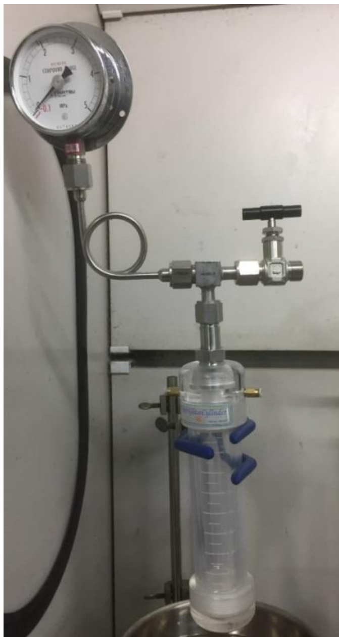
Figure 6. Picture of Thick-Walled Glass Reactor Covered with a Jacket Made of Polycarbonate Used for the Hydrogenation of \gamma -Butyrolactone into 1,4-Butanediol Performed in Table 3 and Scheme 2.
