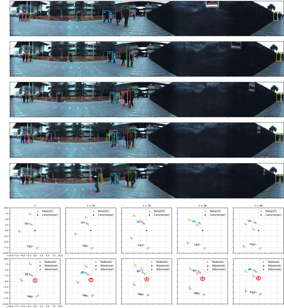
Figure 4.5: Results on real robot dataset. The top four rows show 2D bounding box annotations for pedestrians in the cylindrical RGB image at \tau \in (\tau, \tau + 10, \tau + 20, \tau + 30, \tau + 40) . The fourth row depicts ground-truth global layout of pedestrians relative to the camera x_0 = [0, 0]^\top at every timestep. The fifth row shows the view birdification results given the sequence of 2D bounding box movements in the cylindrical RGB images. Colors correspond to pedestrian IDs. Red triangles denote camera position estimates.
