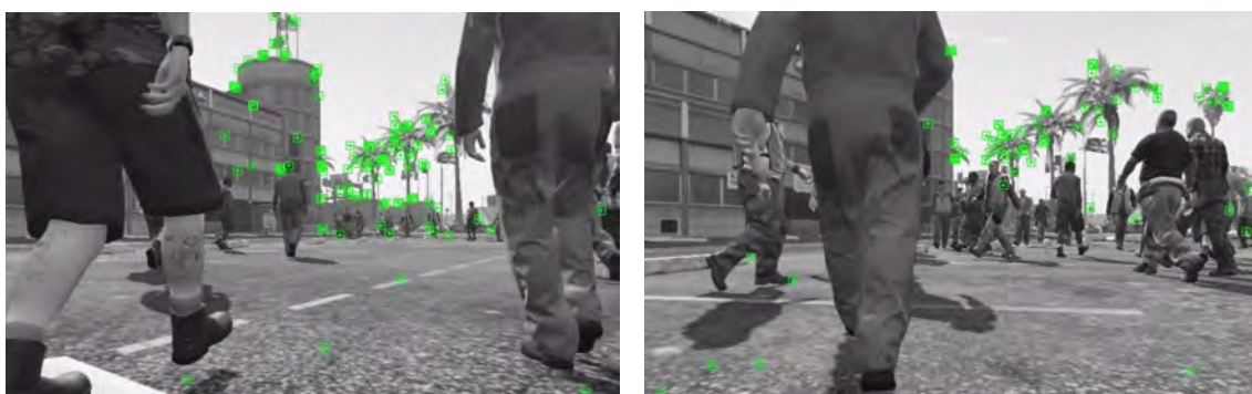
Figure 4.7: Static keypoints trackable in crowded scenes. In these typical two cases, static backgrounds far from the crowd are detected and tracked, while keypoints near the camera are untrackable due to severe occlusions. These static keypoints are at 30[m] from the observation camera.
