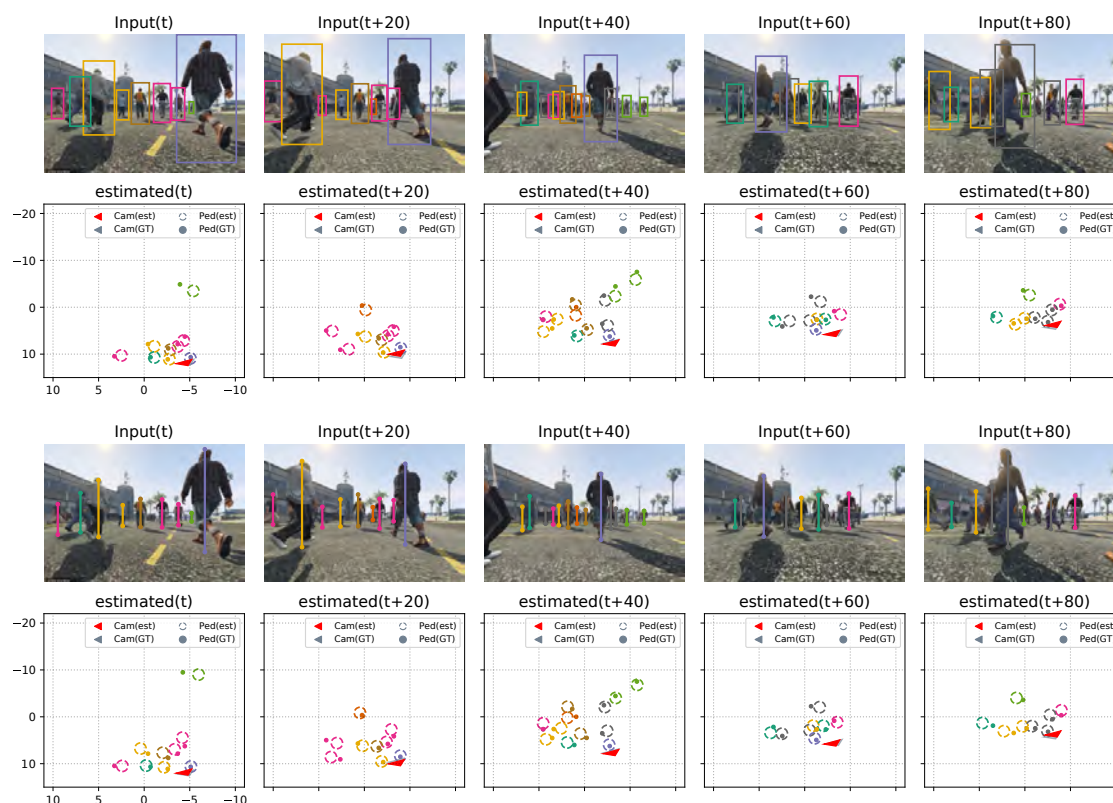
Figure 4.4: Results on photorealistic crowd dataset. The top row shows detected pedestrians with a multi-object tracker in bounding boxes and the third row shows manually annotated human heights (center lines). The figures in the second and fourth rows depict view birdification results for them. Colors correspond to Pedestrian IDs. Red triangles denote camera position estimates x_0^\tau and dashed circles denote estimated pedestrian positions x_k^\tau at time \tau . Grey triangles and circles denote ground-truth camera and pedestrian positions, respectively. View birdification results for both automatic and manually detected people show consistently high accuracy. These results demonstrate the end-to-end accuracy of view birdification.
