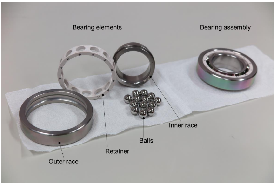
Fig. 4 Self-lubricating ball bearing with glass cloth reinforced PTFE retainer.
