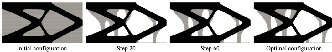
Fig. 3.10 Initial configuration, intermediate results and optimal configuration of cantilever model.
