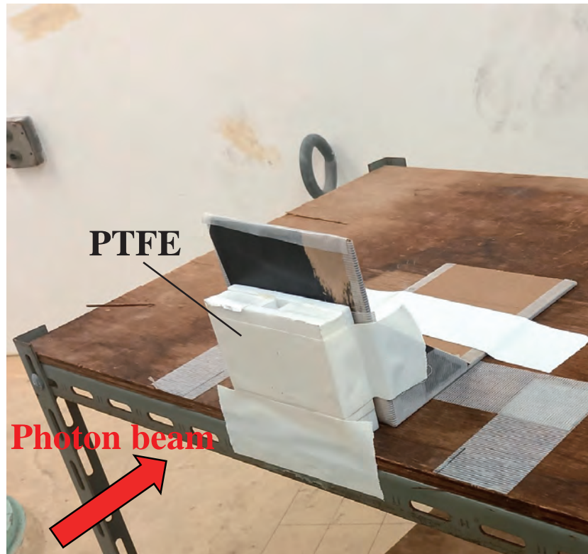
図 3.3.2: Photograph of PTFE plate for the OSLD
