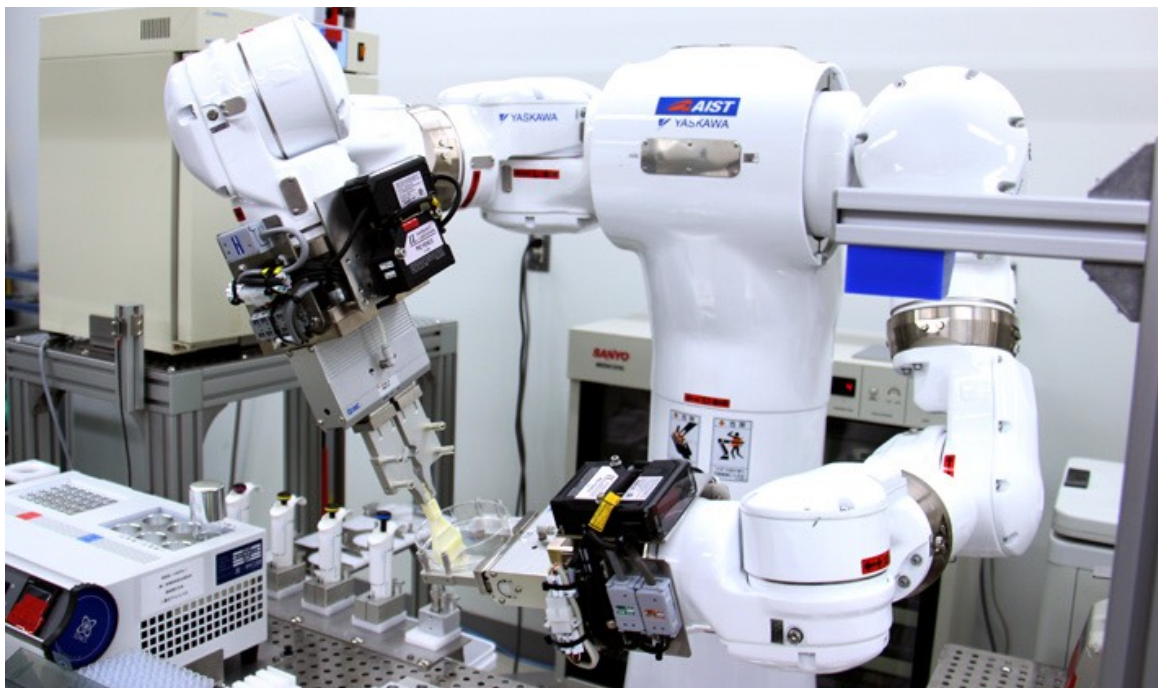
Fig. 5.2 “まほろ,” a robot conducting biomedical experiments developed by National Institute of Advanced Industrial Science and Technology. The proto is quoted from https://www.aist.go.jp/sst/ja/exhibition/innovation_zone/zone11/index.html (accessed 5/21, 2023).
