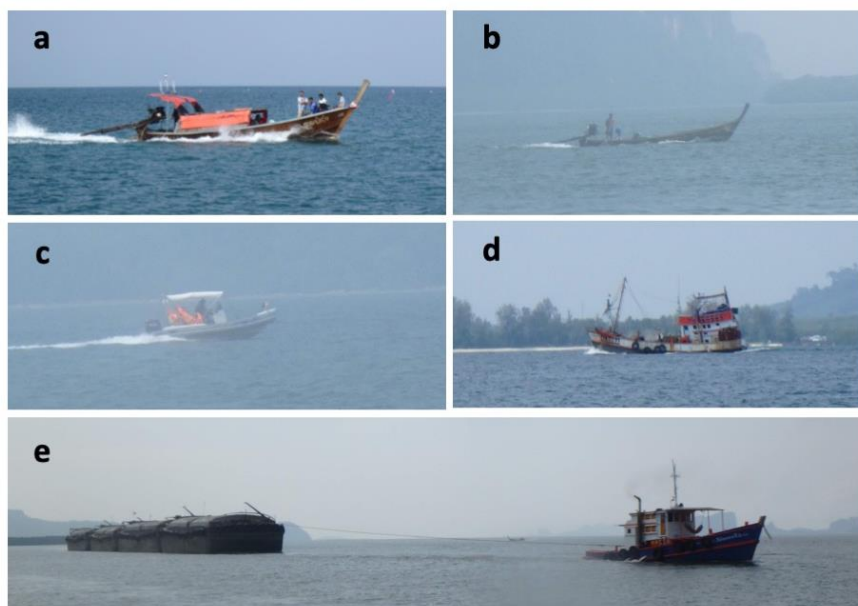
Fig. 2.13 Vessel types visually observed at the monitoring location (Photo courtesy: Kotaro Tanaka). a: Long tail boat, b: Long tail boat (small), c: Speedboat, d: Trawler, e: Tugboat (with
