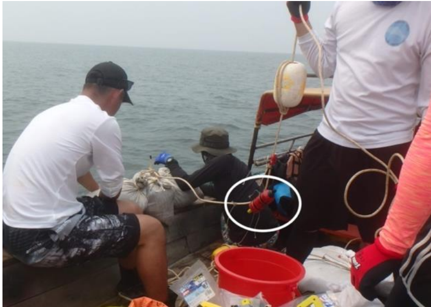
Fig. 3.3 Mooring system of autonomous recorder (Photo Courtesy: Kotaro Tanaka). SoundTrap (marked with white circle) was anchored to two or three sandbags by rope, and maintained upright in the waters by middle and surface buoy. GPS coordinate was obtained right after the deployment.
