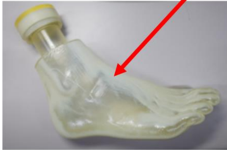
Figure 2.3 Layout for Irradiation test and 3D-printed foot phantom
