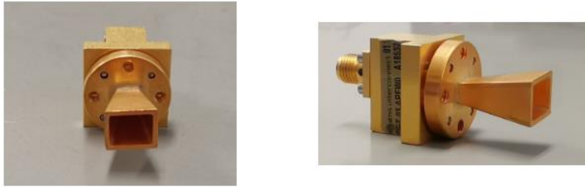
Fig. 4.18 The DET-03 detector. Utilizing Schottky barrier zero-bias diodes, provide the power detection over the 18 to 325 GHz range.
