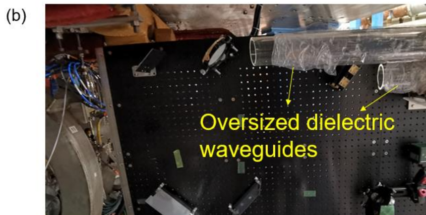
Fig. 4.23 (a) The oversized waveguide on the optical bench A. At the waveguide inlet, the beam size is less than half of the waveguide and the beam waist is located at the waveguide inlet to obtain high transmission efficiency. (b) The oversized waveguide on the optical bench B. Two separate oversized waveguides, one output the probing beam and the other provide the reference beam.
