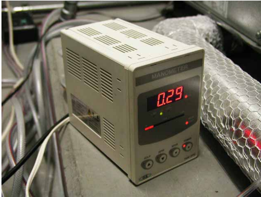
Figure 6.6 Fan pressure head measurement
