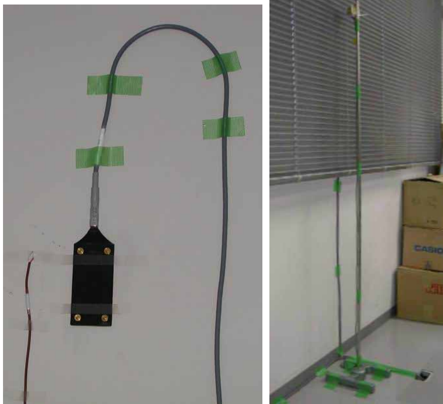
Figure A.5 Measurement of heat flux and solar radiation entering room
