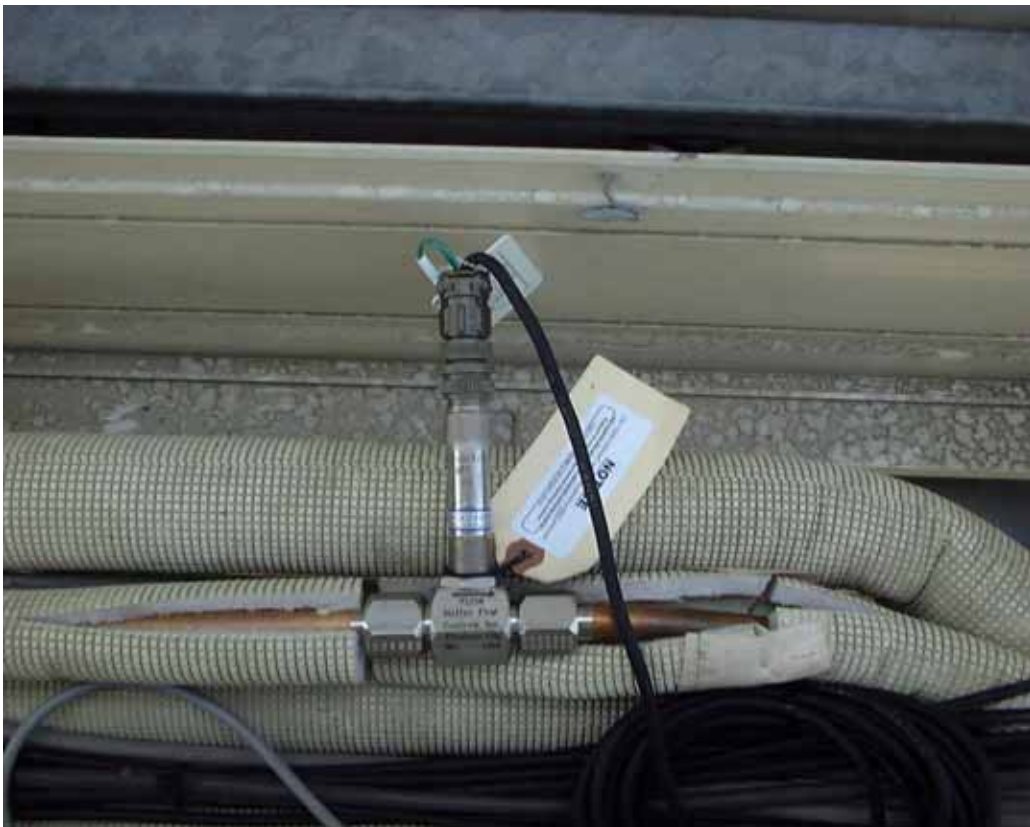
Figure A.11 Measurement of refrigerant flow rate
