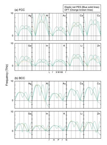
FIG. 6. (Color online) Phonon dispersion relationships for ten elemental metals with (a) fcc and (b) bcc structures. Phonon dispersion curves obtained by the elastic net PES and DFT are shown by blue solid and orange broken lines, respectively. Negative values indicate imaginary modes.
