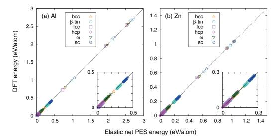
FIG. 5. (Color online) Comparison of the energies predicted by the elastic net PES and DFT for (a) Al and (b) Zn, measured from the energy of the most stable structure among the bcc, fcc, hcp, sc,  $\omega$  and  $\beta$ -tin structures.
