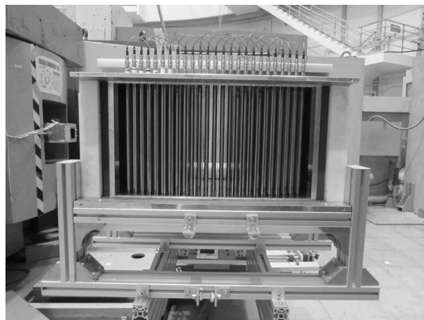
Fig. 2. Twenty-five 3 He tube detectors (1/2 inch in diameter) on the detector bank.
