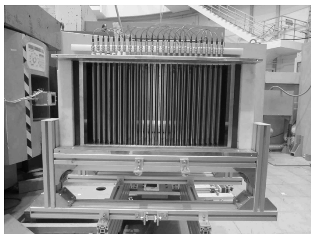
Fig. 2. Twenty-five 3 He tube detectors (1/2 inch in diameter) on the detector bank of the VCND.
