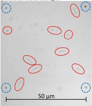
Fig. 1. Microscopic image of the detector after development. Observed tracks are surrounded by red ellipses. Marks for fine alignment are surrounded by dashed blue circles. Tracks and marks were clearly seen after development.
