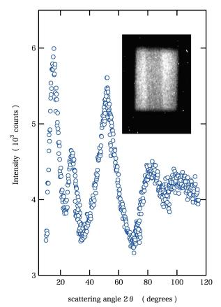
Fig. 1. Neutron diffraction patter of the borosilicate glass for vitrification without simulated radioactive waste recorded on the B-3 diffractometer. The inset shows a neutron transmission image for the same sample.
