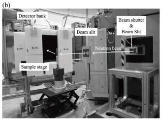
Fig. 1. Versatile compact neutron diffractometer (VCND) installed at the B-3 beam port of Kyoto University Research Reactor (KUR): (a) bird's-eye-view photograph and (b) partial view (around the sample stage) of the VCND.
