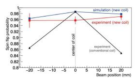
Fig. 3. Position dependence of spin flip probability.
