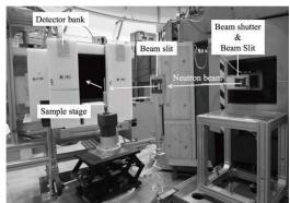
Fig. 1. Versatile compact neutron diffractometer (VCND) installed at the B-3 beam port of Kyoto University Research Reactor (KUR).
