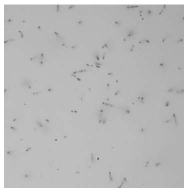
Fig. 1. One of the microscopic images of the detector that recorded tracks of \alpha particle and {}^7\text{Li} from neutron absorption by {}^{10}\text{B} . The dimension of field of view was 50\times 50\ \mu\text{m}^2 . About 120 tracks were recorded in this area by 1000 seconds of neutron irradiation.
