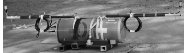
Fig. 2. Appearance of AUSOMS-D. The figure shows the pressure-tight case and the hydrophones.
