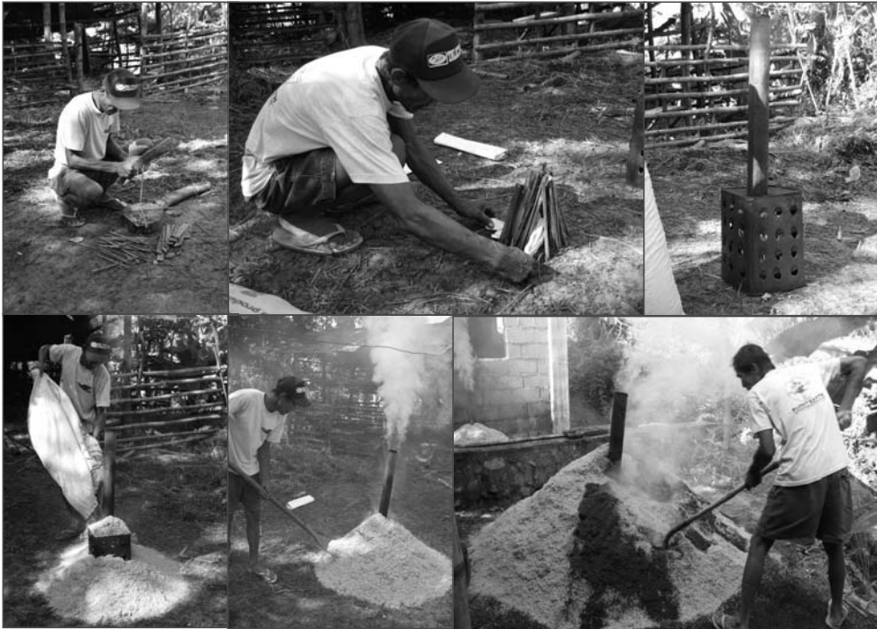
Fig. 5 Process of carbonizing rice hull. From top left: cutting small twigs as fuel and starting the fire; a hand-built carbonizer; pouring sacks of crude rice hull around the carbonizer; turning over the rice hull heap to ensure even heat distribution
