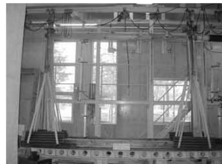
Fig. 12 Strength test of a rib-frame
