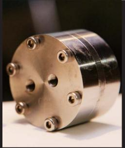
This tiny device fits snugly into the palm of a hand. Any two reactant chemicals passed through it can be made to mix perfectly and instantaneously. Small quantities of agents are sufficient for this process, making it energy efficient and eliminating waste. Mae dreams of a time when this technology might be widely used in small, local chemical production facilities, replacing today's huge production plants that consume vast amounts of energy and resources and generate hazardous waste.
