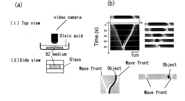
Figure 1: Experimental results on transportation of a piece of paper. (a) Experimental system. (b)Spatio-temporal plot for directional intersection at the broken line in the upper picture. The bright and dark regions correspond to the oxidized and reduced states, respectively.
