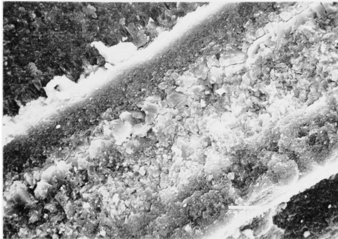
Fig. 7. Scanning electron micrograph showing concentric laminations of crystallized substances in the mid-zone. Reduced from \times 2,000 .
