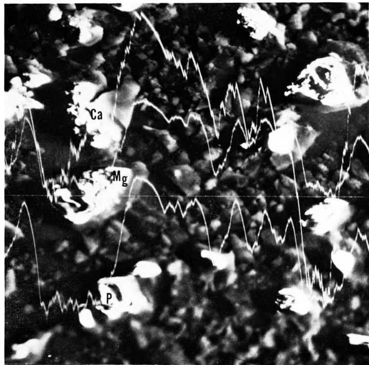
Fig. 3. A small amount of Mg as well as Ca and P are still detected in another apatite calculus. The upper curve is that for Ca-K \alpha , the middle curve Mg-K \alpha and the lower curve P-K \alpha . The three curves have almost the same pattern. \times 1,700
