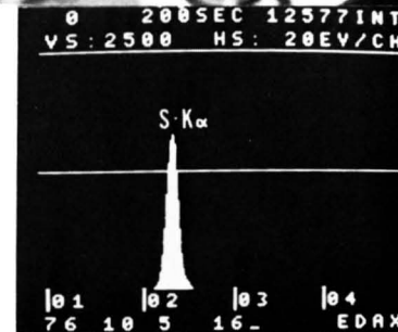
Fig. 8. Image and analysis of control cystine. Only S is detected. \times 1,700
