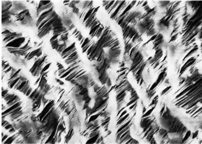
Fig. 1. Scanning electron micrograph of IMPRA graft ( $\times 2000$ ).
