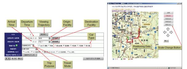
Figure 2. Web-diary system with probe trajectories (Tanabe et al., 2007)
