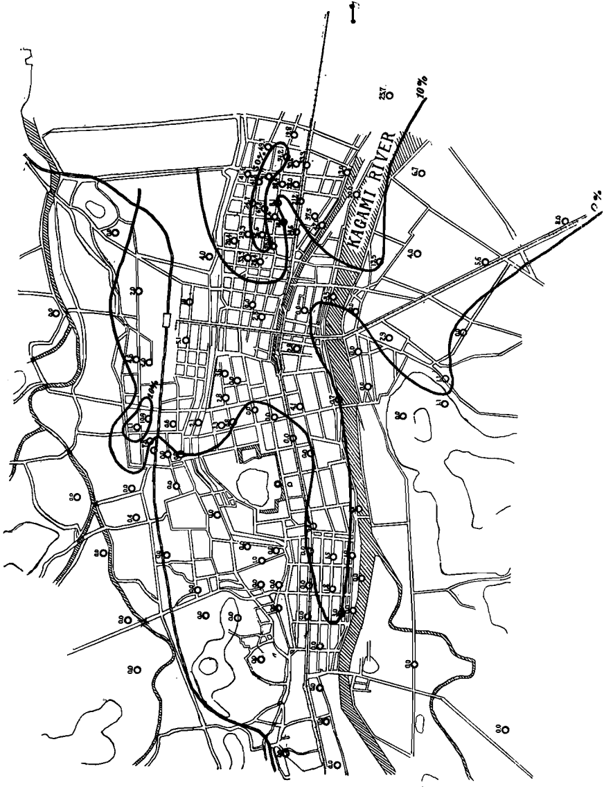
Fig. 23 The rate of complete damage at Kōchi.
