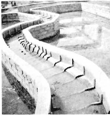
Photo. 2. Model channel with artificial roughness.
